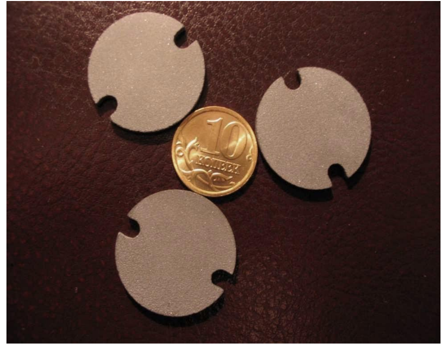
Photo of heat spreading plates made of IKRAM material
